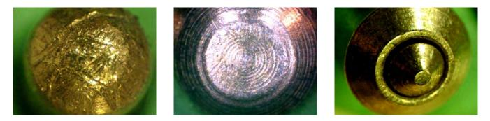
The marks left by an attacker are in many ways indicative of their skill level. In this photo (left), deep and plentiful pick marks are shown. The attacker, an amateur, used extreme force on both tension and pick tools. The extreme tension causes pins to bind against plug and require more force to be lifted.
