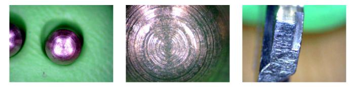
New pins are clean, with no dust, grease, or dirt. Light abrasions and corrosion may exist depending on how the pins were stored prior to being used in the lock. Factory original pins usually do not exhibit these characteristics. A clear indication that pin has not been used is the fresh milling marks around the tip of the pin.
