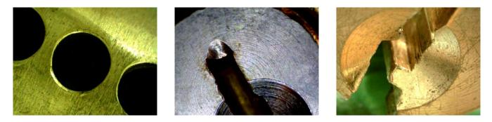
The pin chambers within the plug may also be damaged by bumping. When kinetic energy does not properly transfer to the top pin, the pin stack may instead press against the chamber walls (caused by the movement of the bump key). Repeated bumping may cause these areas to distort, stretching in various directions. In the photo (left), the pin chamber is stressed is distorted in many directions, but mostly to the top left.
