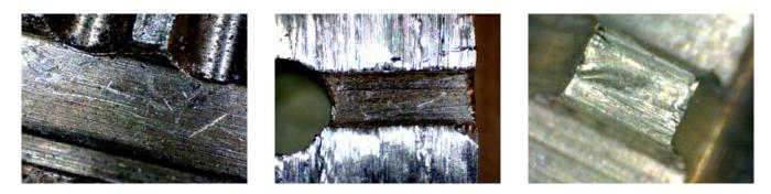
Inside the plug we also expect to find various forensic evidence. In this photo (left), the plug walls have scratches are various angles that are inconsistent with the use of a key.
