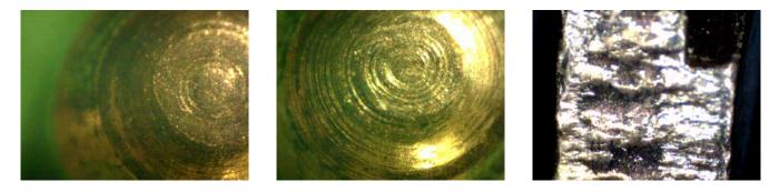
At 1,500 uses (roughly 1.5-2 years of use) a distinct change in the appears of the pins. The key has been used so many times that the milling marks have almost completely been removed. Again, slight scratches on the pin are being caused by the key becoming more jagged as it too wears down.
