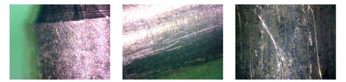
For the attacker, it is difficult to not touch the sides of pins. This can happen during raking as well as single-pin picking. Marks left on the sides of pins are quite noticeable and not as prone to wear and those in the center of the pin. In the photo (left), light scratches at varied angles are visible.
