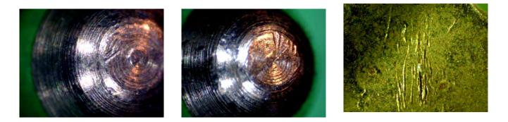
The striking of the pick gun needle against the bottom pins causes very clear forensic evidence. Unlike picking, which causes scratches, the pick gun causes impact marks that, when done many times, begin to resemble the spokes of a bicycle along the circumference of the pin. In this photo (left), several impact marks are visible.
