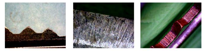
Possession of keys that are made by hand are, in a general sense, somewhat suspicious. In most cases hand made keys are easily identified by measuring the ramp angles, shoulder to first cut distance, and the distance between cuts. Hand-made keys generally have imperfect, jagged ramp angles and poorly spaced cuts.
