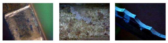
Various materials are transferred to the key during use. Generally hair, fiber, and fingerprints will be examined by a crime lab. The forensic locksmith, however, may examine the findings of the crime lab to identify the uses of materials found on keys. In this photo (left) we see a light green residue, which happens to be modeling clay.
