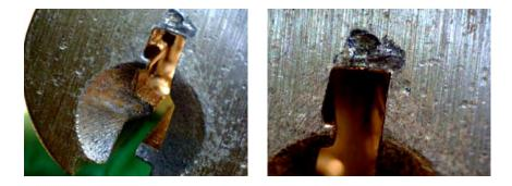
The face of a lock that has seen moderate to heavy use will have many dents and imperfections caused by normal use. How many times have you went to unlock a door and slightly missed the keyway? In the photo (left), many small dents and scratches from normal use are visible.
