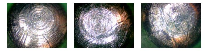
The act of using a pick tool is invasive, and we expect the stronger material of the pick tool to cause marks on the softer brass or nickel-silver of the lock components. In the photo (left), we see scratches where the pick tool was used to lift the pin. These appear to be single-pin picking marks due to their shape, size, and position.
