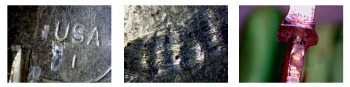
Sometimes marks will be left on the key as a result of normal or malicious use. When a key is duplicated with a cutter, the clamp to hold the original or the blank may leave a mark. In addition, some covert entry techniques may leave tool marks. In this photo (left) we see a set of rather deep marks on the bow.
