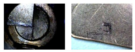
Cam manipulation is one of the most common bypass methods. The American 700 (old models) suffer from this vulnerability. Essentially, the cylinder is not required to move in order to actuate the cam. In the photo (left), tool marks left on the cam and back plate indicate that bypass was used as the method of entry.
