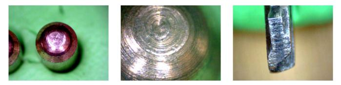
After 250 uses (roughly 3-6 months of use) a ring develops around the pin. This is the key gliding under the pins, spread around the tip because insertion and removal lightly rotates them back and forth. The key is also lightly polishing the pins, too.
